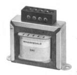
Dimensions 4" x 21/2" x 3" high. Weight 2 lb. Fixing holes 3 1/8" P.C.D. Maximum input 15 watts. Frequency response ±1dB 30 to 20,000 c/s. D.C. Resistance of Primary 375 ohms (185 and 190 ohms each half) Inductance at 8 v. A.C. (no D.C.) 100 H. Leakage Inductance .085 H.
