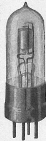
The Edison A.R. Bright Emitter valve. The corresponding Dull Emitter of this make (A.R. '06) can be used in the set described.
